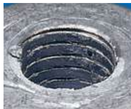
Defective thread
