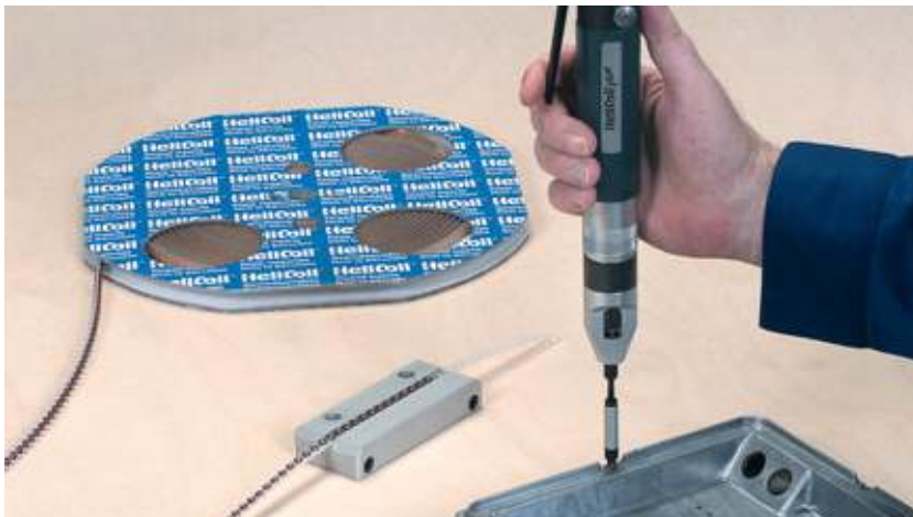
Installation of HELICOIL® Plus
